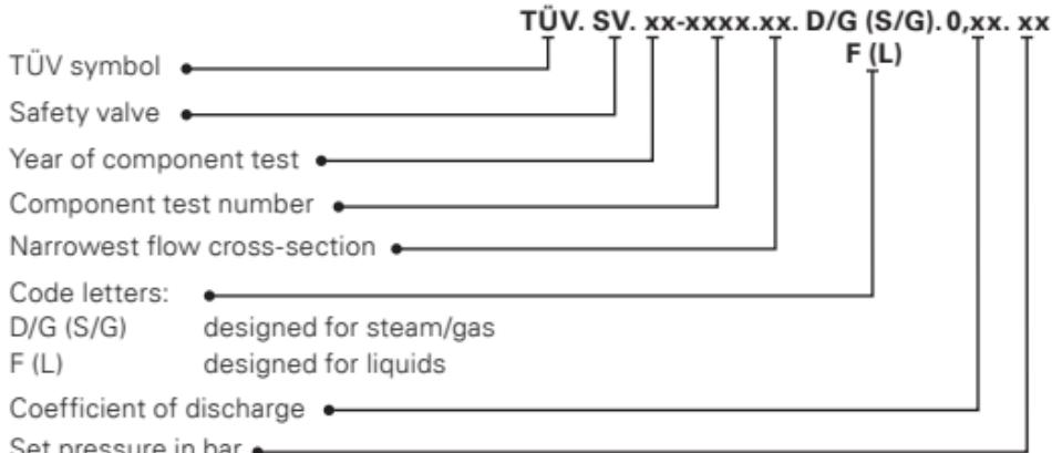
We check the safety valves for pressure resistance and tightness, adjust the requested set pressure and seal them. The identification on the type plate or on the spring bonnet of the valve is applied using a permanent marking system. In addition markings and technical data according to DIN EN ISO 4126-1 are included on the identification plate.
